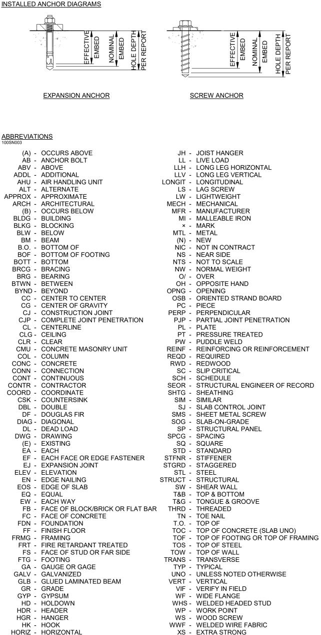
HORIZ - HORIZONTAL XXS - DOUBLE EXTRA STRONG HSB - HIGH STRENGTH BOLT HSS - HOLLOW STRUCTURAL SECTION Ø - ROUND OR DIAMETER HT - HEIGHT
